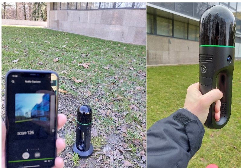
Figure 4: Scanning process in the field with handheld laser scanner the Leica BLK2GO
