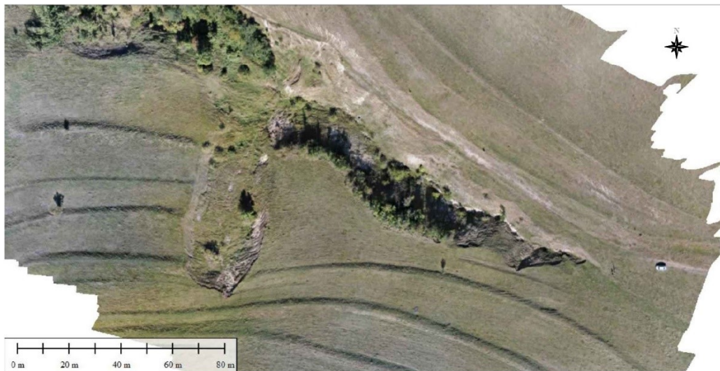
Figure 6. The orthophoto map (1:2000) resulted from the first drone flight above the surveyed area.
