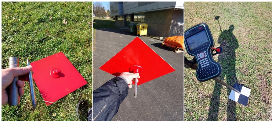
Figure 3: Ground control points – technical solution and GNSS measurements
