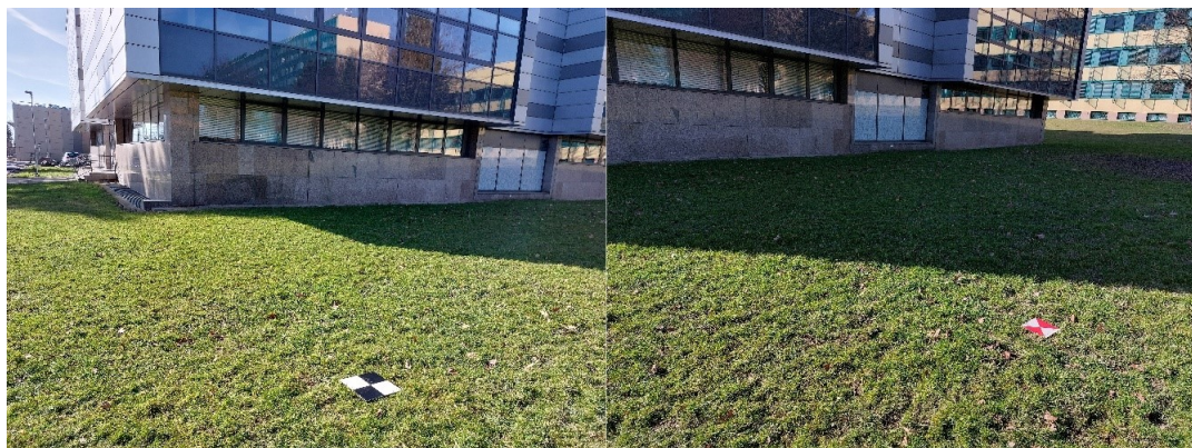
Figure 2: Type of ground control points
