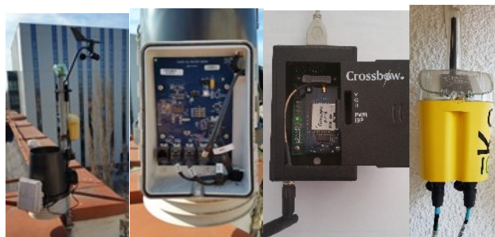
Fig. 1. The micro-weather station, the radio-base and a wireless node.
