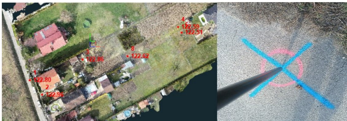
Fig. 2: Configuration (left) and marking (right) of GCPs.
