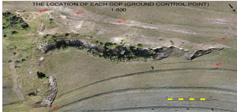
Figure 2. The location of each GCP (Ground Control Point ) with red colour
