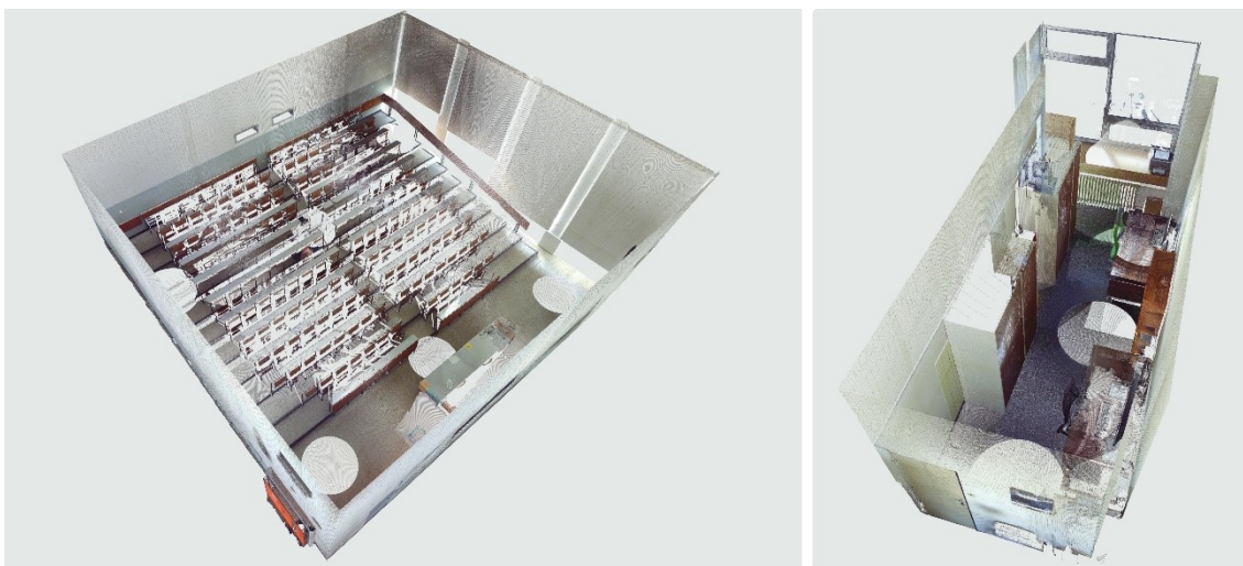
Figure 3: The point cloud from TLS of the third (left) and the fourth (right) evaluated building space
